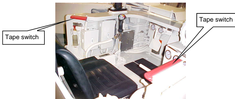
Fig. 46: Tape switch (panic strip) location
