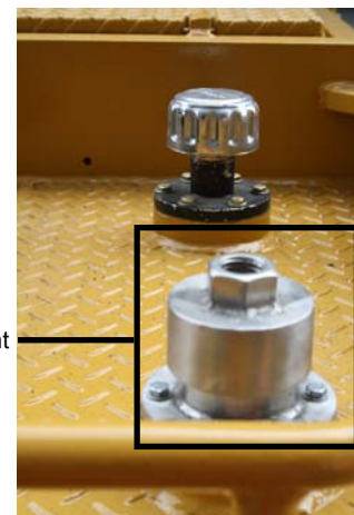
Hydraulic Tank Fill Point
