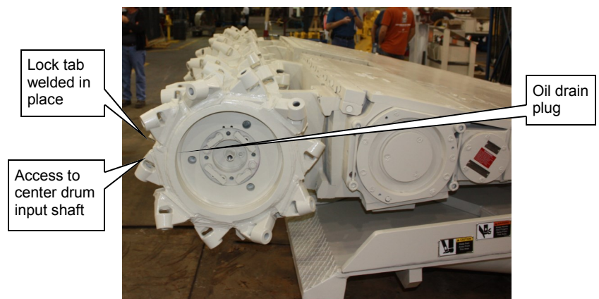
Fig. 160: Lock tabs tack welded to capscrews
