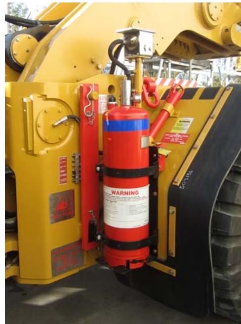
FIRE SUPPRESSION SYSTEM
