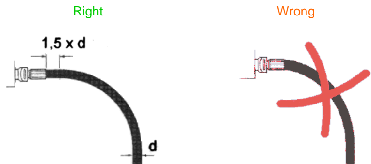
Fig. 3: Laying hydraulic hoses, bending
