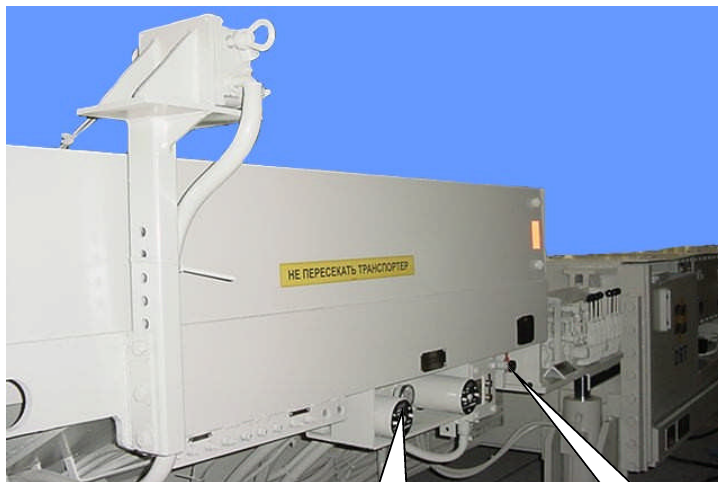
Fig. 16: Shutdown control (s) locator
