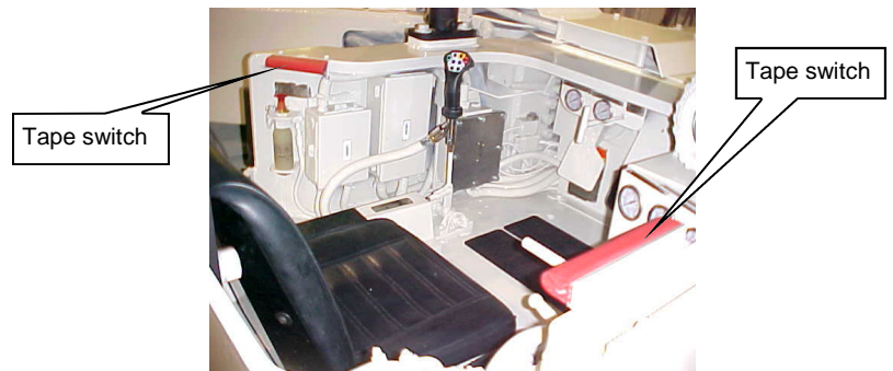
Fig. 36: Tape switch (panic strip) location
