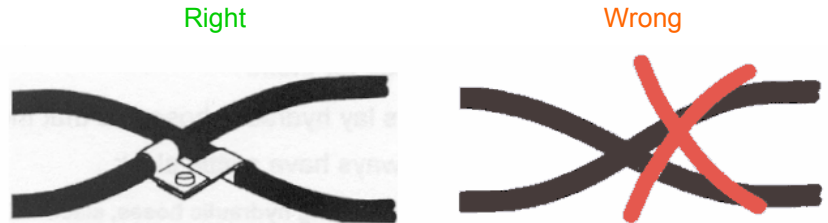
Fig. 5: Laying hydraulic hoses, crossing
