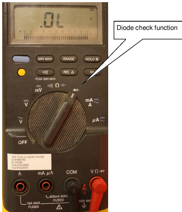
Digital multimeter with diode check function
