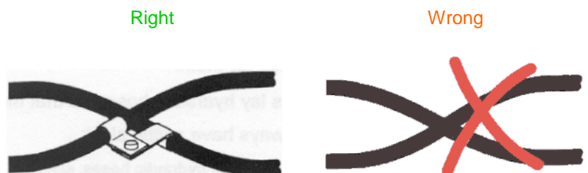
Fig. 4: Laying hydraulic hoses, crossing
