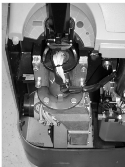
Figure 3.21. Drive unit and main transmission fixing bolts
