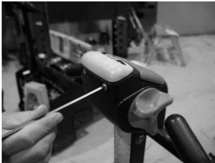
Figure 4.8. Main fixing screws at the back of the tiller arm head assembly
