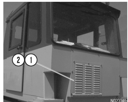
FIGURE 40-4. 1. Filter Cover 2. Cab Filter
