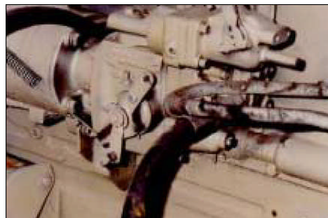
Fig. 105: Cummins PT fuel system
