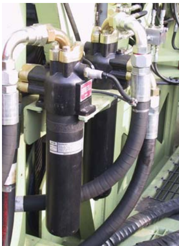
Fig. 4-9 Hydraulic Loop Filter—Two filters mounted on each side of mast "A" frame.
