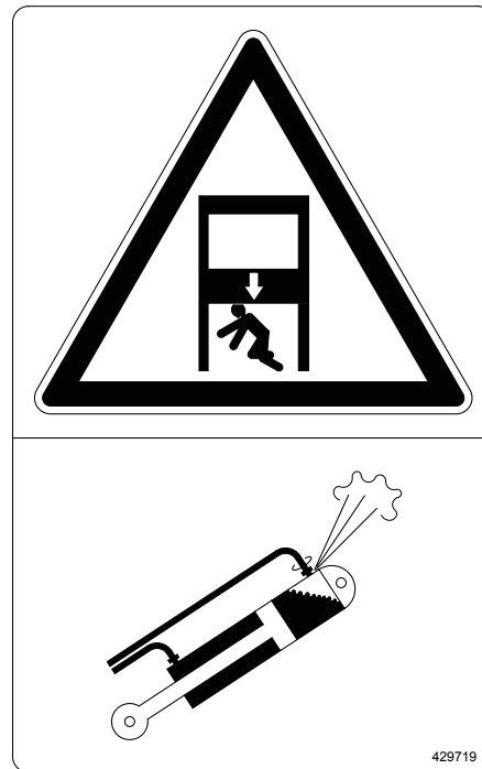
Crush Hazard–Rotary Head (429719)
