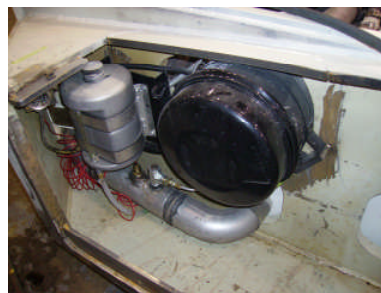
Fig. 69: Typical intake system
