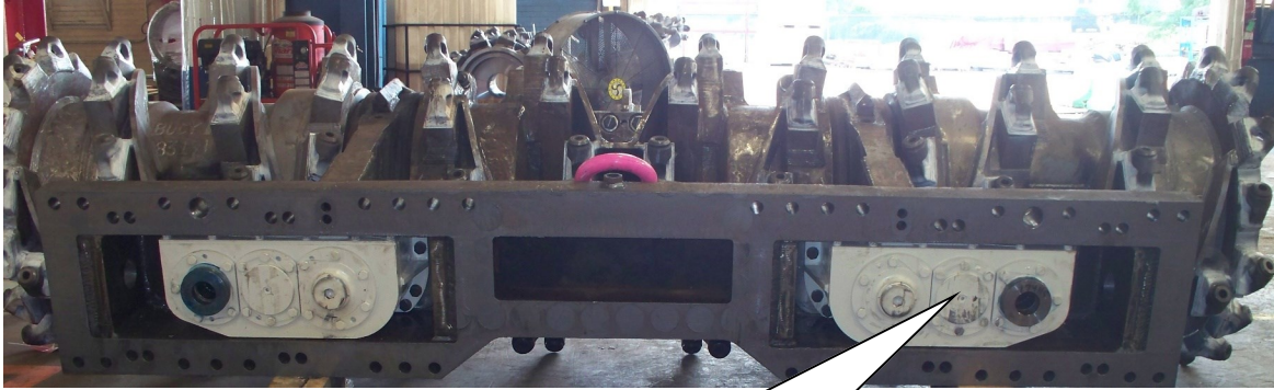
Fig. 126: Gear case breather locations
