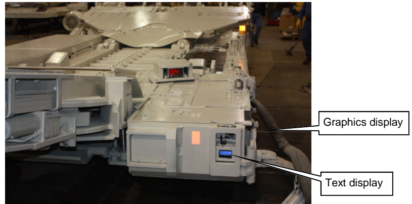
Fig. 17: Control system display locations (typical)
