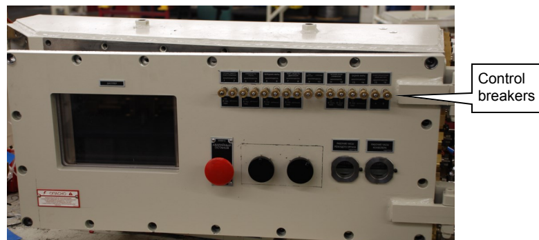
Fig. 65: Operator's case - control breakers
