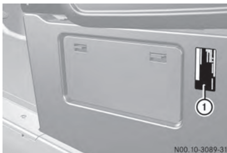
Vehicle identification plate for vehicles or chassis on the base of the driver's seat
