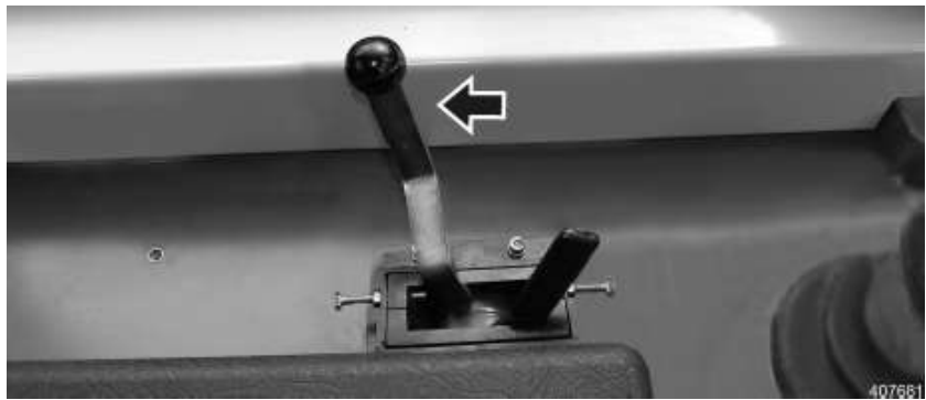
Throttle control lever – low idle
