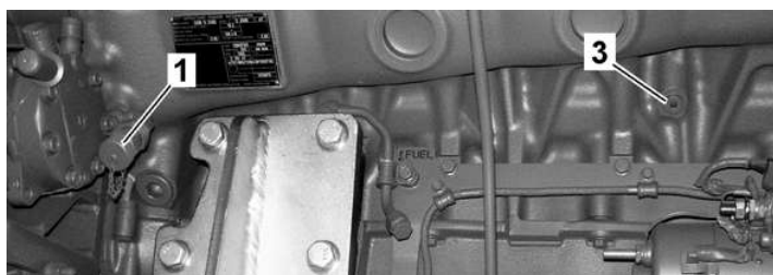
Fig. 5-28 Coolant draining valve and screw on engine front side
