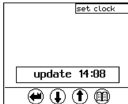
Fig. 3-29 Confirmation of the storage of the new time
