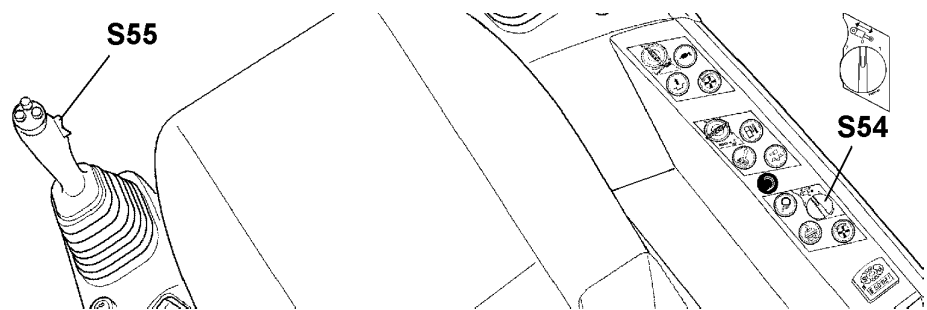
Fig. 3-103 Switch for the unlocking of attachment movements cut off
