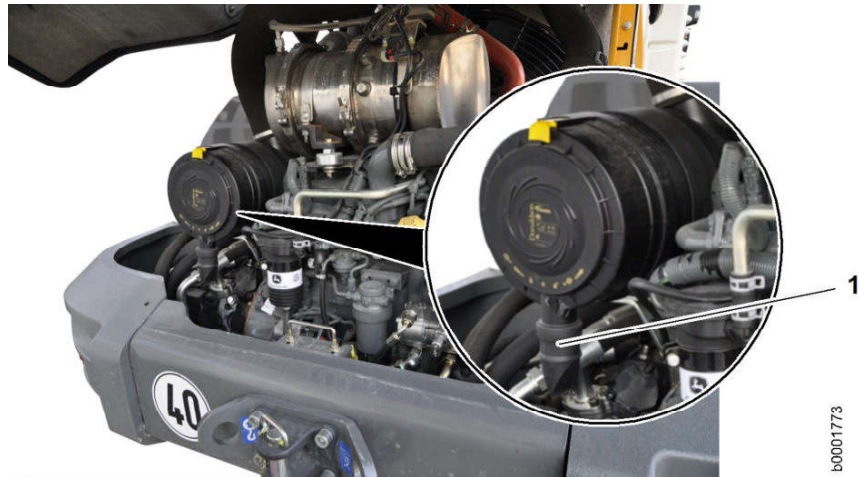
Fig. 337: Cleaning the dust discharge valve
