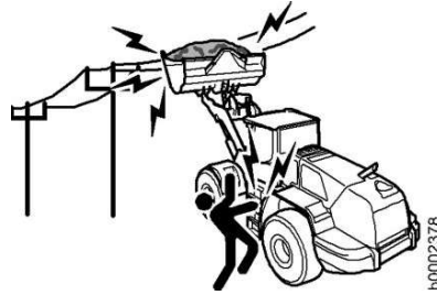
Fig. 265: Working near overhead power lines
