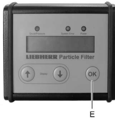
Fig. 253: Diesel particulate filter control unit in the driver's cab:
