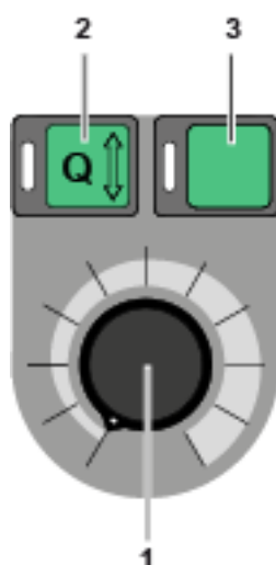
Fig. 1197: Control unit Feed speed on control panel X25 (only for slow gear)
