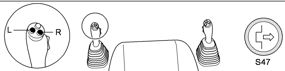
Fig. 3-109 Releasing and locking of coupling system by means of push buttons*
