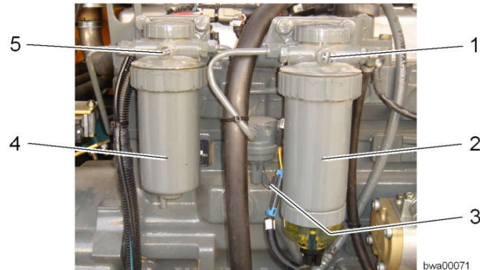
Fig. 440: Bleeding the fuel filter
