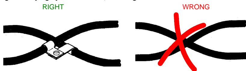
Fig. 5: Laying hydraulic hoses, crossing
