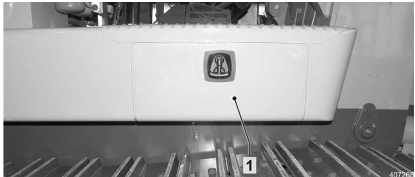
Access – refueling pump
