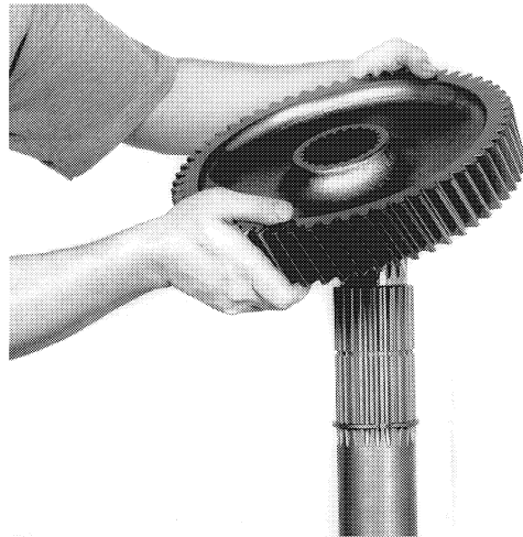
Figure 63 Position output gear on shaft with long hub of gear toward inner ring.
