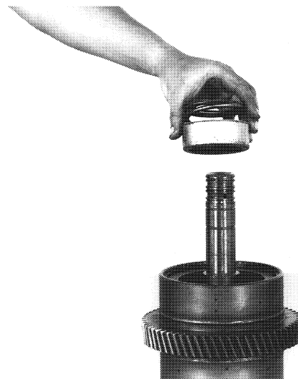
Figure 244 Compress piston return wave spring. Remove return spring retainer ring. Remove ring retainer, wave spring and spring retainer.
