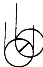
Not adjusted properly. (Needs Shims.)
