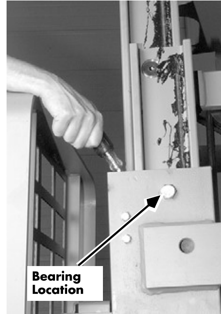
Figure 7-250: Upper Mast Bearing, Main Mast
