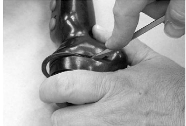
Figure 7-38: Control Handle Retaining Ring Removal (EZ/ES/ET/EF)
