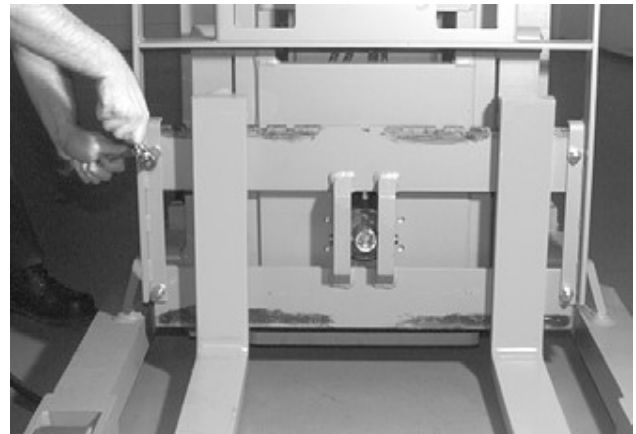
Figure 7-269: Fork Removal (with Tilt and no Sideshift)
