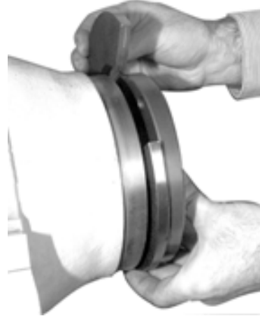
Figure 6-96: Remove Seal Tool Halves
