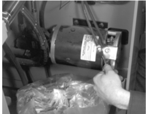
Figure 5-105: Remove the Power Cables
