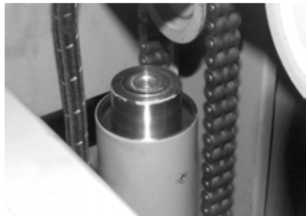
Figure 7-57: Piston Cap Removed
