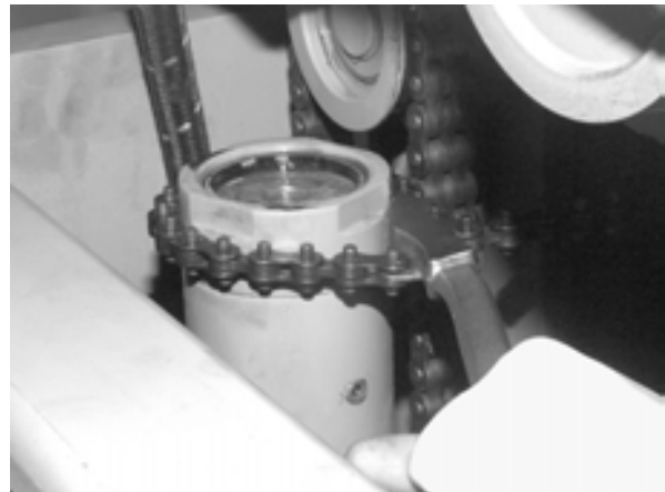
Figure 7-56: Remove Piston Cap
