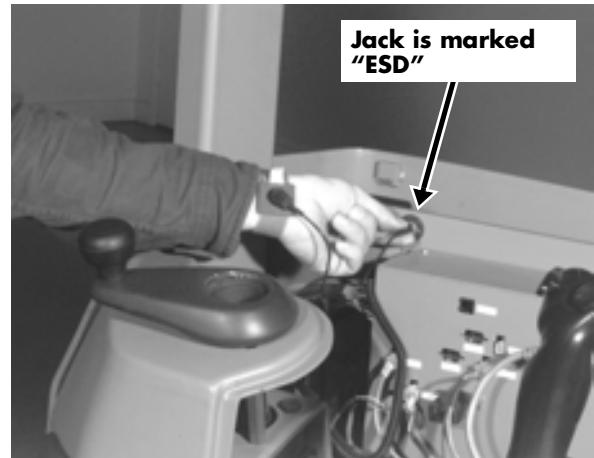
Figure 5-148: Attaching the Static Discharge Wrist Band and Plugging It In
