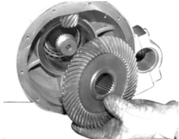
Figure 6-97: Install Spiral Bevel Gear
