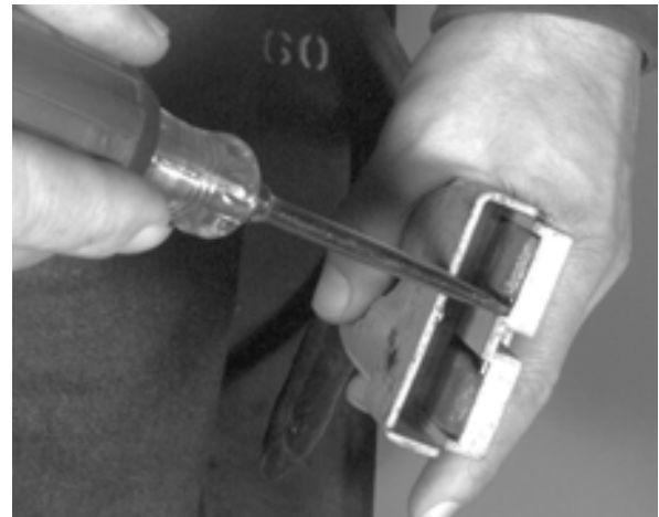
Figure 5-21: Removing Cable from the Battery Connector
