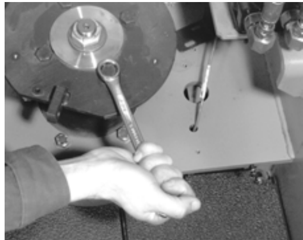
Figure 6-74: Install Steer Plate Bolts
