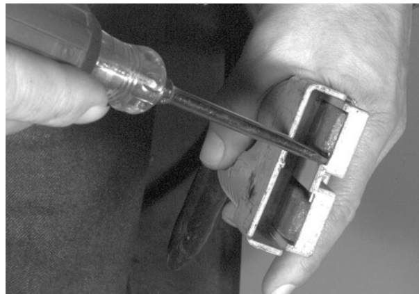
Figure 7-34. Battery Cable Removal from Connector
