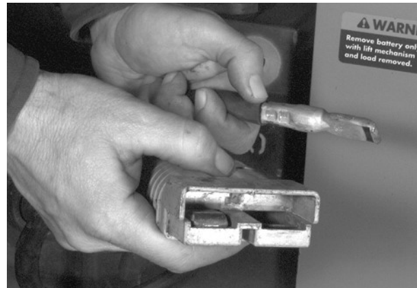
Figure 7-34. Battery Cable Removal from Connector
