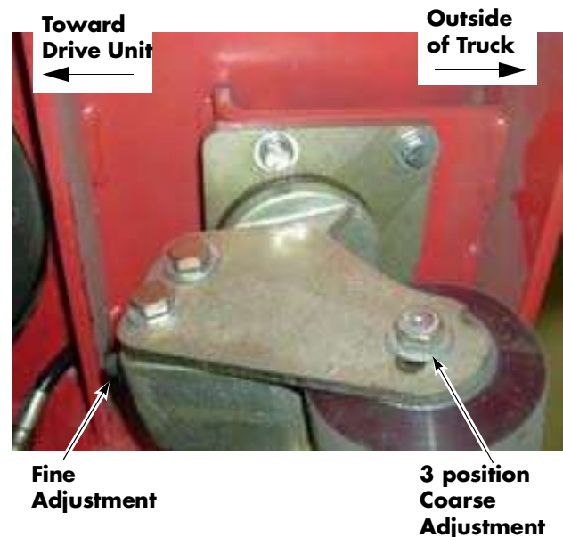
Figure 7-43. Adjustable Caster Adjustment
