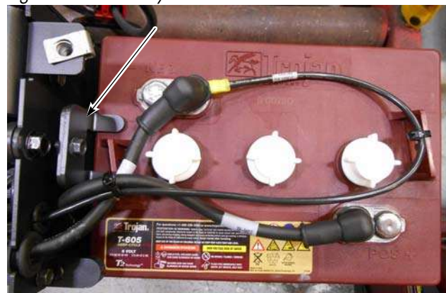
Figure 7-51. Battery Retention Bracket Installed
