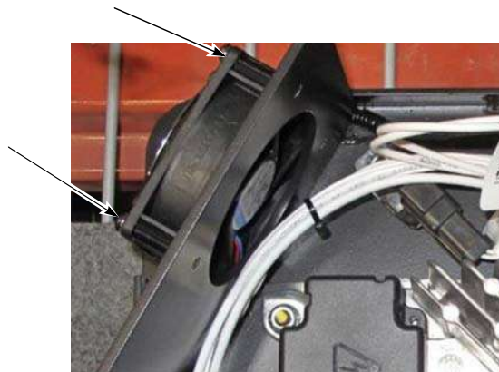
Figure 7-76. Fan Mounting Screws
