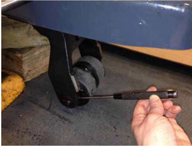
Figure 7-121. Removing Spiral Pin
