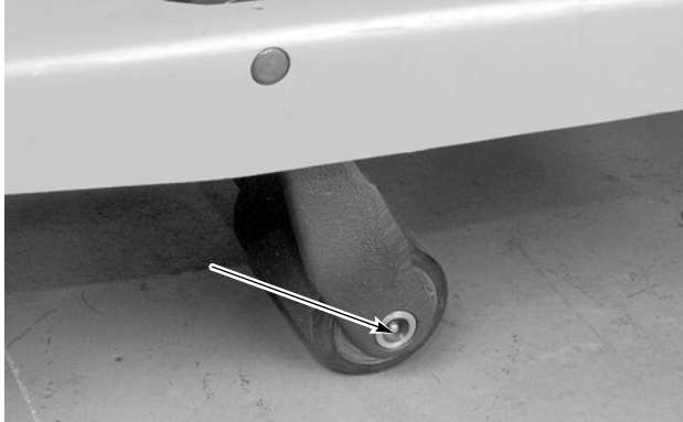
Figure 4-1. Load Wheel Axle (Single Wheel)
