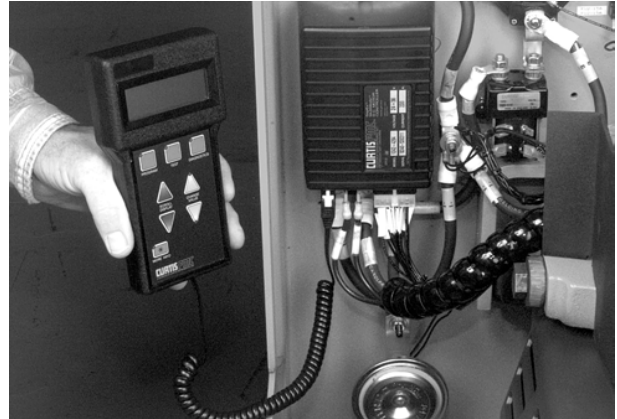
Figure 5-6: Connecting the PMT to the Motor Controller
