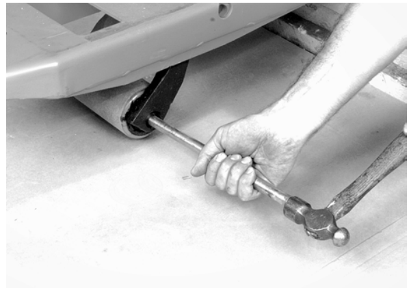
Figure 6-49: Removing Axle From Load Arm Casting
