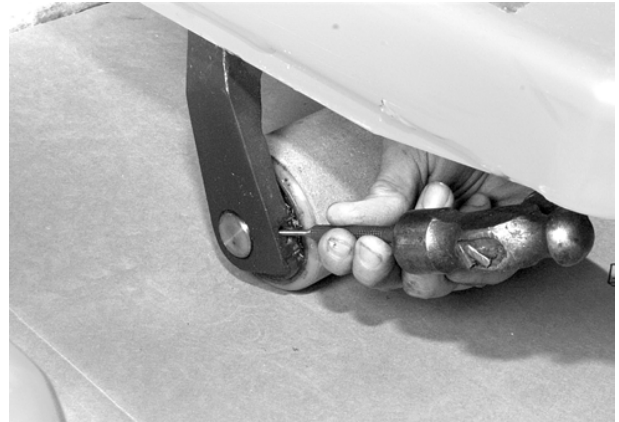
Figure 6-48: Removing Tension Pin
