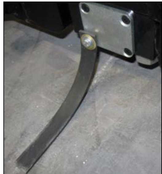
Figure 4-5 ESD Strap Location
