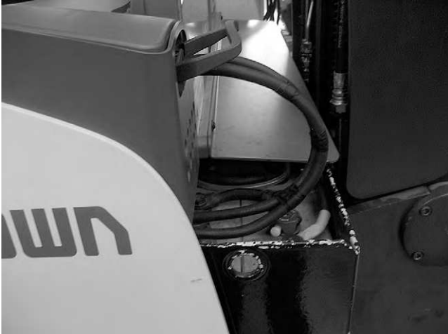
Fig. 133 840 Ah: battery retracted
