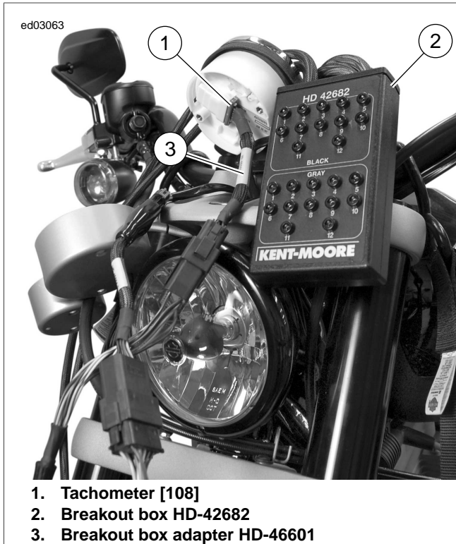
Figure 1-25. Breakout Box Connection (XR)
