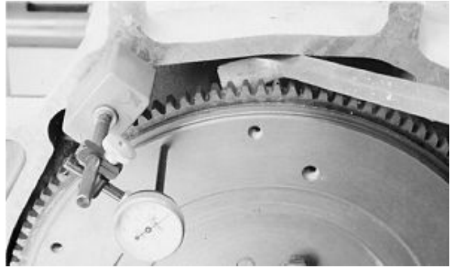
Check Crankshaft End Play w/Dial Indicator
