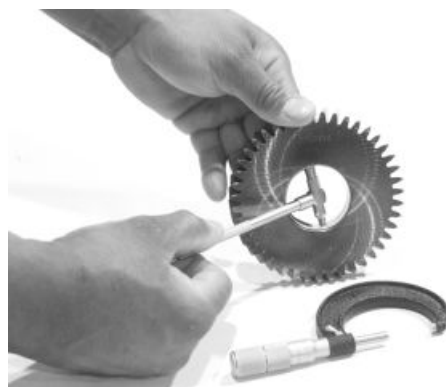
Measuring Idler Gear Bushing ID
