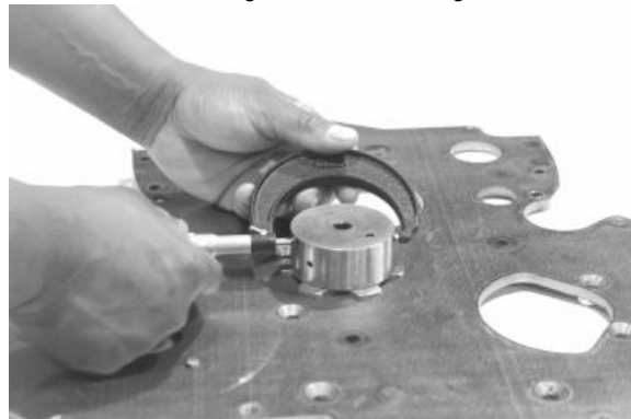
Measuring Idler Shaft Journal OD
