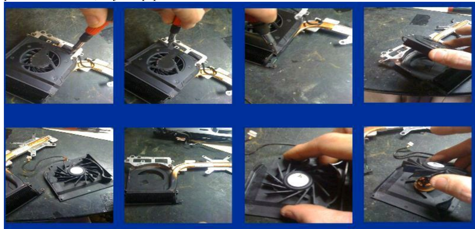
More Pictures of Fan/Heat-Sink Cleaning
