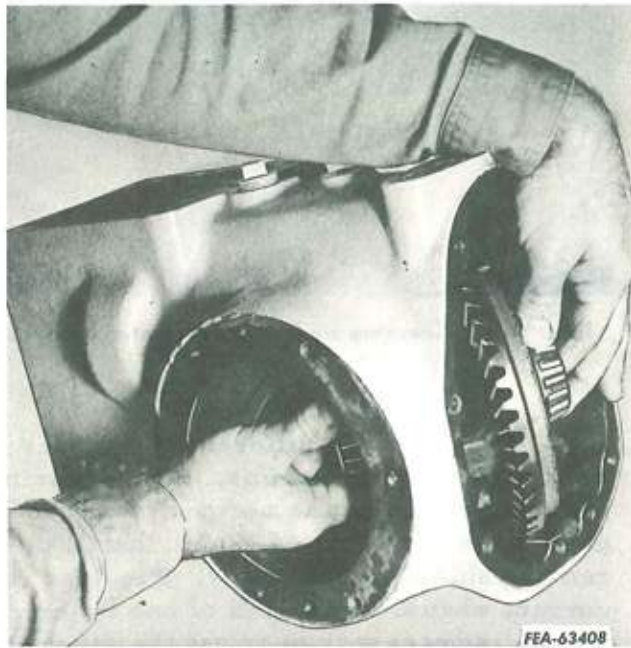
Illust. 2-41. Removing differential from the transmission case.
