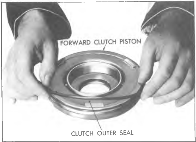
Fig. 71T—Removing Forward Clutch Piston Outer Seal
