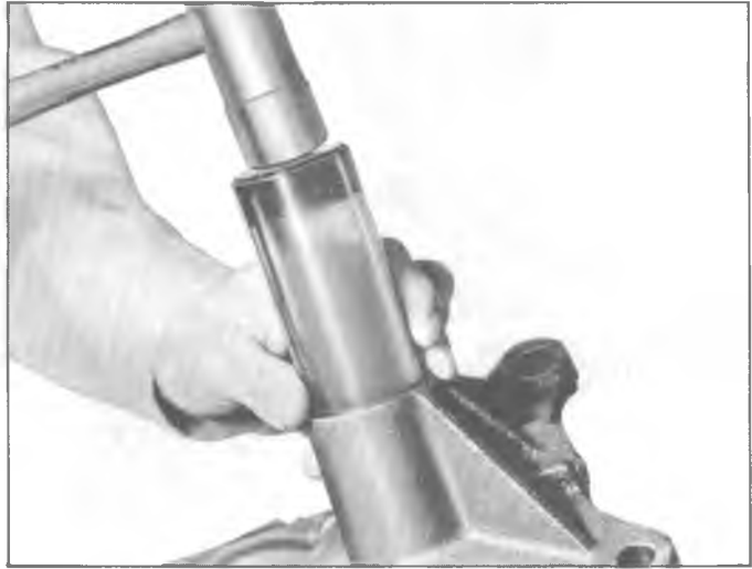
Fig. 14—Installing Sector Shaft Seal Using Installer Tool J-9225
