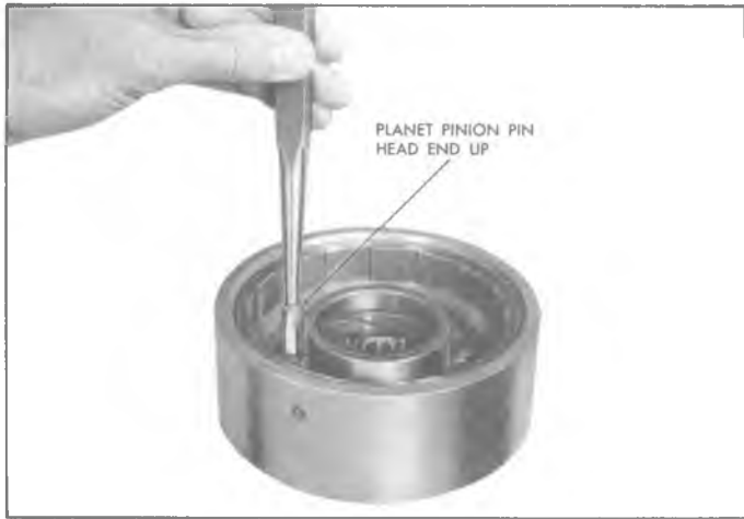
Fig. 109T—Installing Planet Pinion Pin
