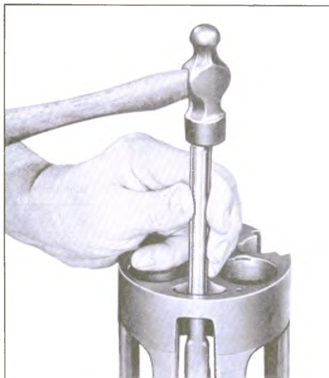
Fig. 18—Unseating Discharge Crossover Tube
