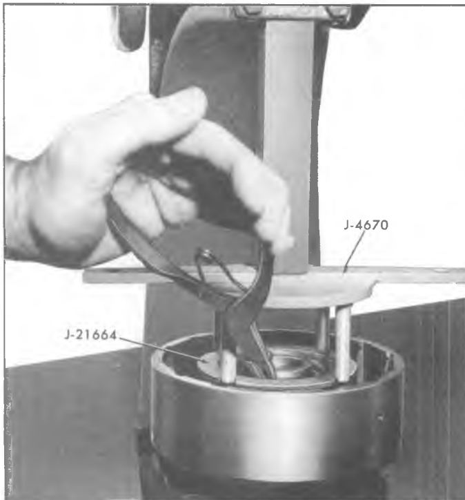
Fig. 70T—Removing Forward Clutch Spring Retaining Snap Ring
