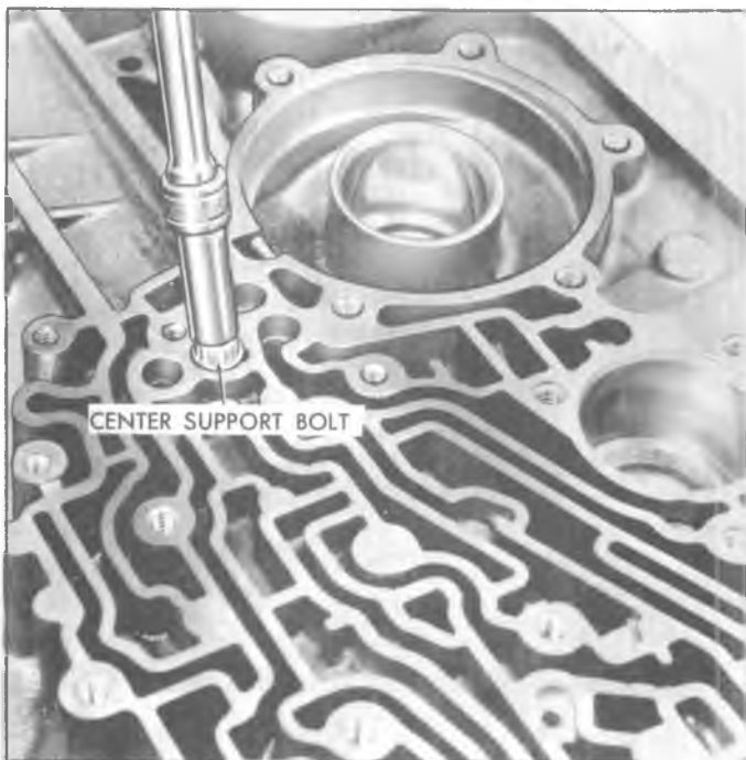
Fig. 33T—Center Support Locating Bolt
