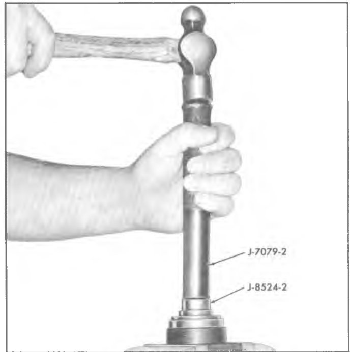
Fig. 72—Removing Needle Bearing and Seal
