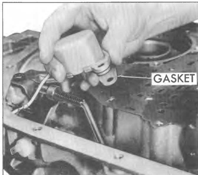
Fig. 144T—Installing Detent Solenoid and Gasket
