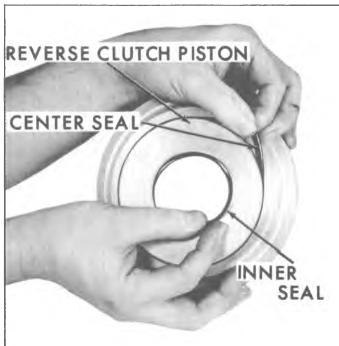
Fig. 52M—Removing Low and Reverse Clutch Piston Center and Inner Seal
