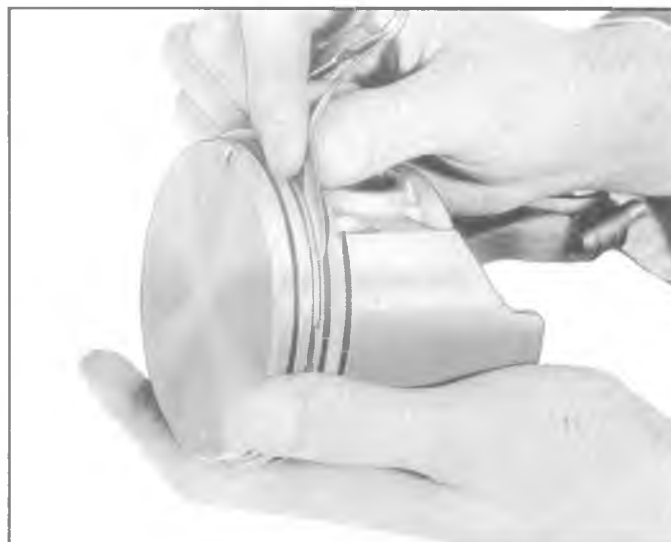
Fig. 56—Checking Ring in Groove
