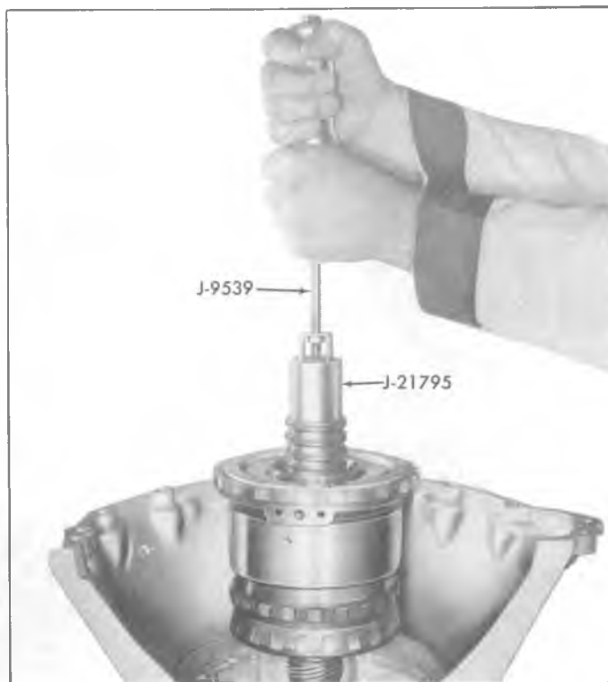
Fig. 36T—Removing Case Center Support and Gear Unit from Case
