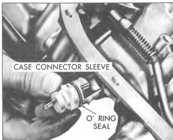
Fig. 145T—Installing Case Connector Sleeve and "O" Ring
