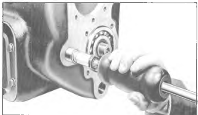
Fig. 3S—Removing Idler Gear Shaft
