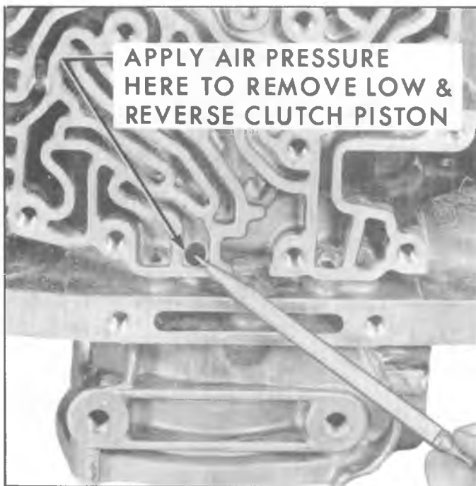
Fig. 50M—Removing Low and Reverse Clutch Piston
