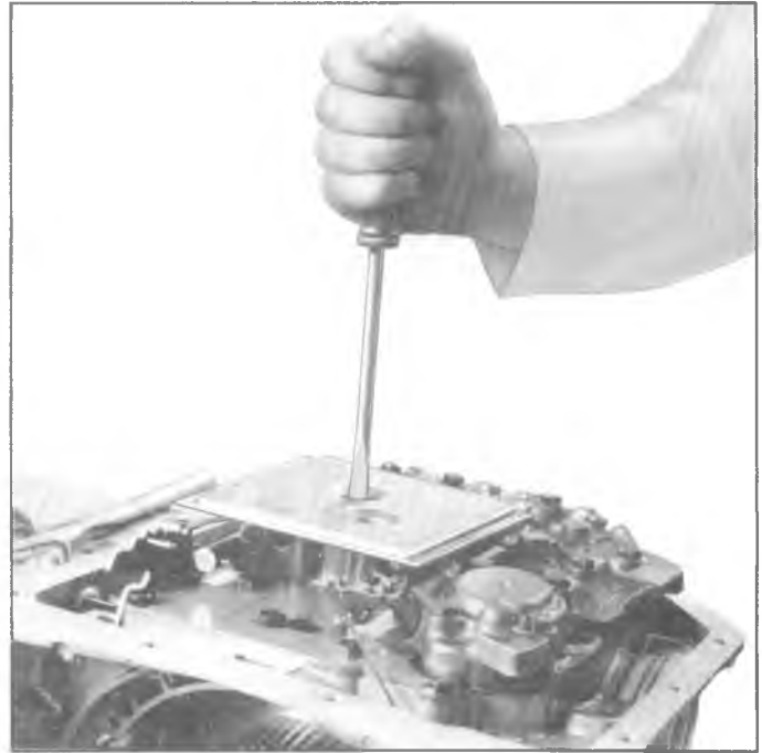
Fig. 12M—Removing Oil Pump Strainer From Valve Body
