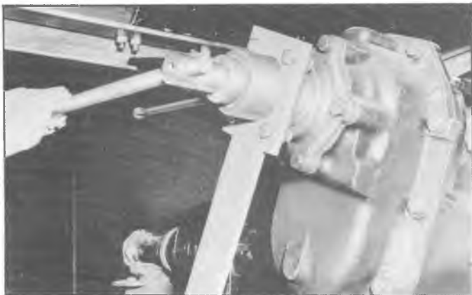
Fig. 101—Removing Input Shaft Flange Nut
