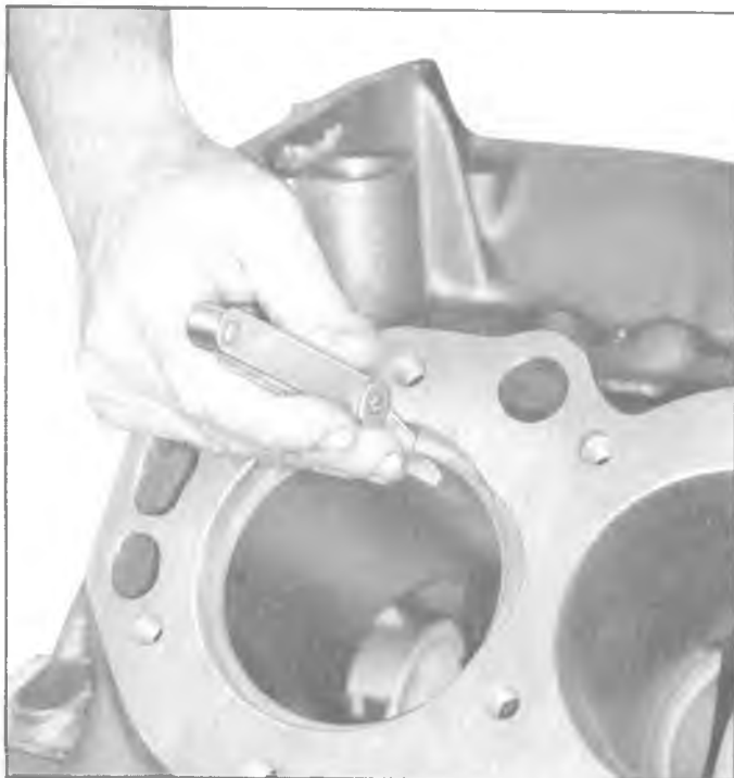
Fig. 55—Measuring Ring Gap
