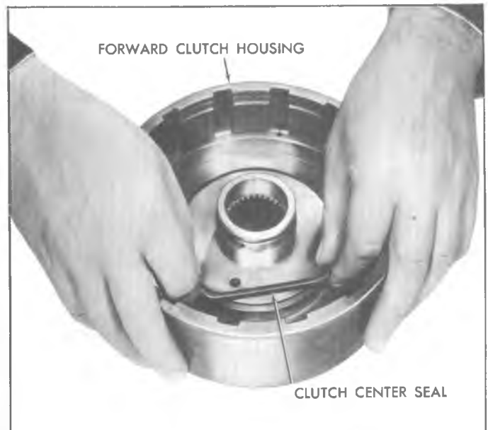
Fig. 72T—Removing Forward Clutch Center Seal
