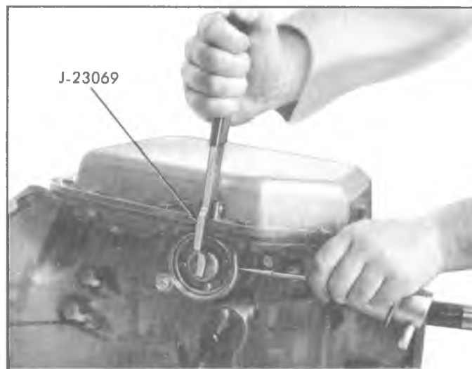
Fig. 53M—Removing 1-2 Accumulator Piston Cover
