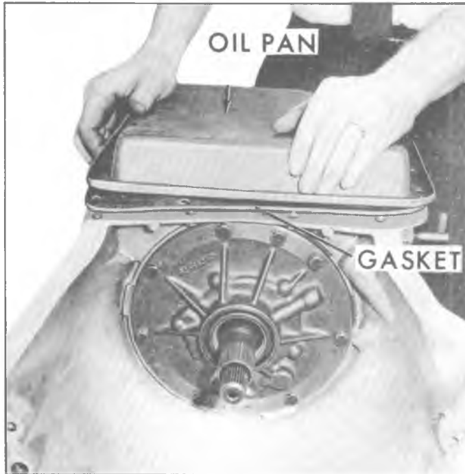
Fig. 11M—Removing Transmission Oil Pan
