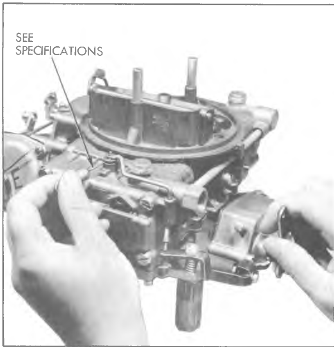
Fig. 17H—Air Vent Valve Adjustment
