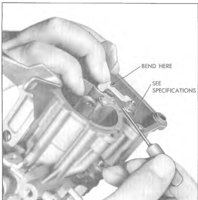
Fig. 5R—Metering Rod Adjustment
