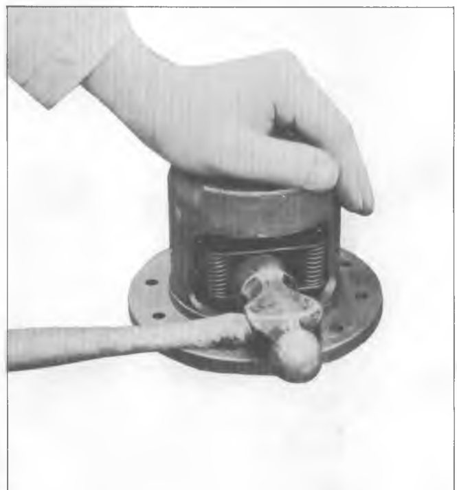
Fig. 35—Installing Spring Pack
