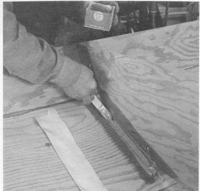
The resin has been applied to a short frame-mold seam, and the glass putty is going on with a tongue depressor. Fiberglass tape is cut and ready. The resin-filled brush will be used to smooth the tape in position over the freshly filled seam.
