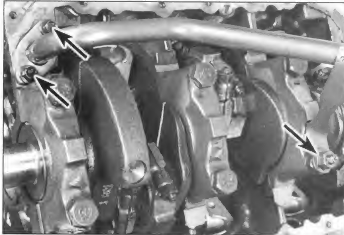
15.11 To detach the V6 engine pickup tube, remove the nut and bolt (arrows)
