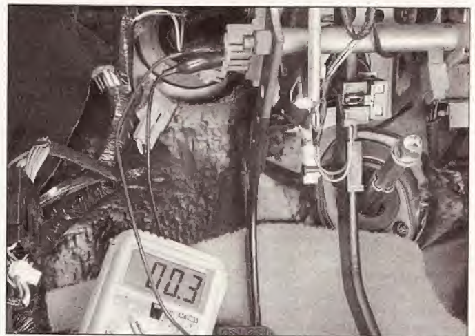
7.4 To check the operation of the switch, unplug the switch electrical connector and hook up an ohmmeter to the terminals for the red and light blue and the pink and white wires; with the clutch pedal released, there should be no continuity, but when the pedal is depressed, there should be continuity (shown)
