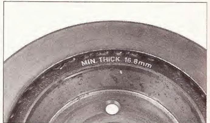
5.6a The minimum thickness limit is cast into the inside of the disc
