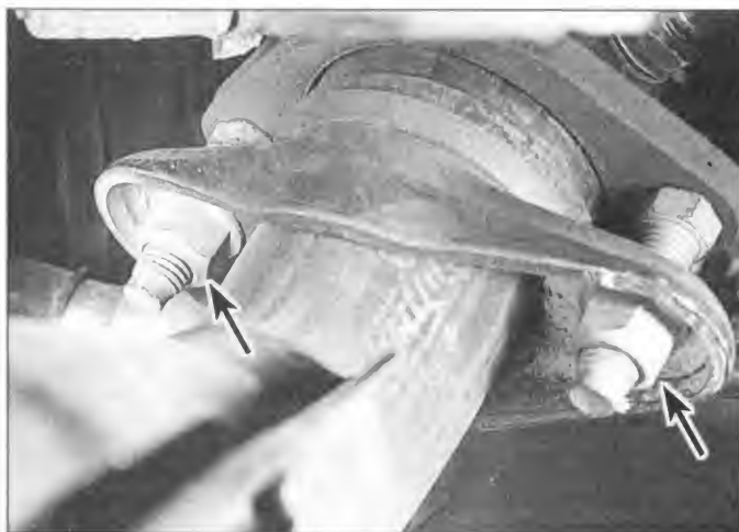
8.5 From below, remove the two exhaust pipe-to-manifold nuts (arrows)
