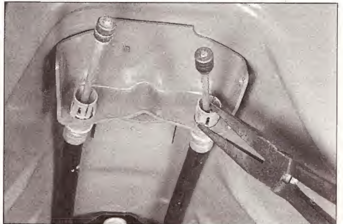
10.12e ... then squeeze the tangs of the cable housing together and disengage the cable from this bracket
