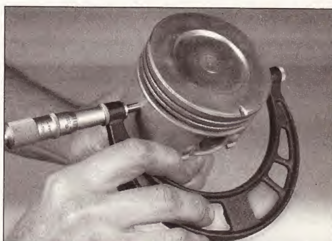
18.11 Measure the piston diameter at a 90-degree angle to the piston pin and in line with it
