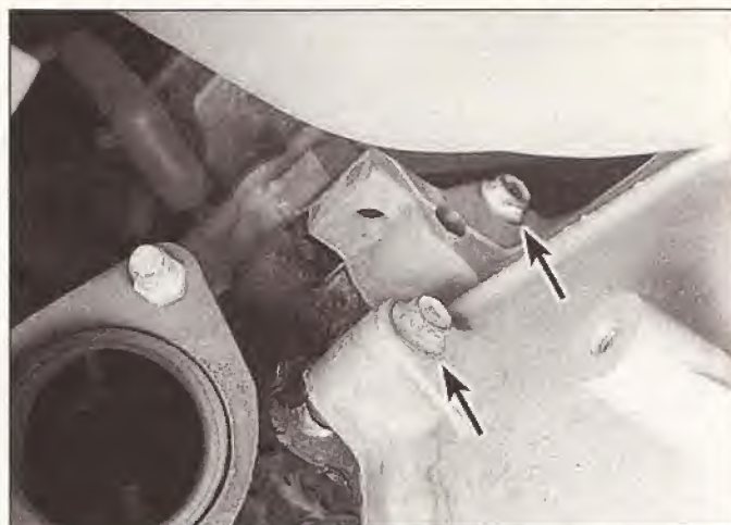
6.18a Remove the bolts (arrows) securing the left side of the transmission bellhousing to the engine
