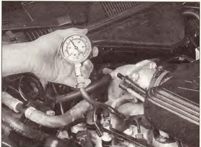
3.7 If you don't have the correct adapter, it is possible to remove the Schrader valve from the fitting and install a standard fuel pressure gauge, using a hose clamp (4.6L SOHC engine shown)
