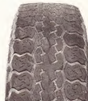
FEATHERING DUE TO MISALIGNMENT
