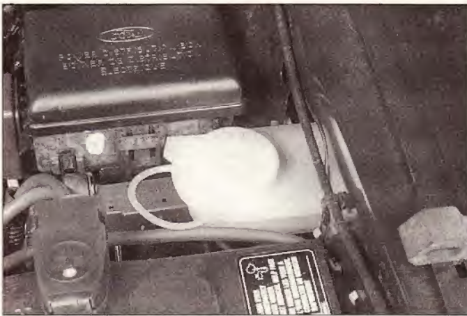
4.22 The windshield washer reservoir is located at the left front corner of the engine compartment next to the battery
