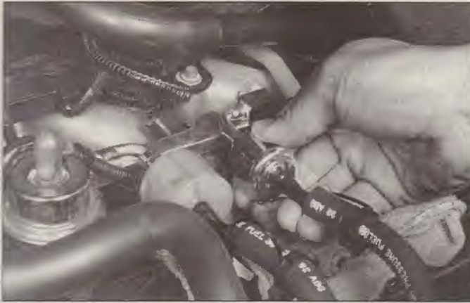
13.36a Press down to release the safety clamp from the fuel line connectors
