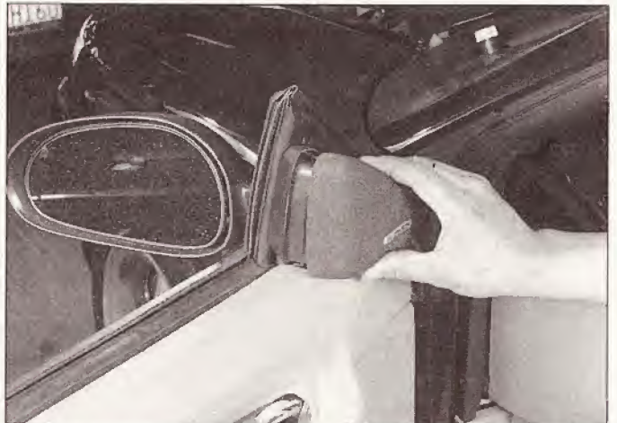
17.6a Pull straight out to remove the side view mirror trim cover or speaker cover (if equipped)
