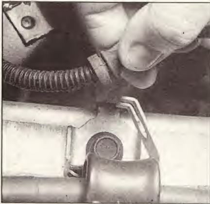
9.2 If the vehicle is equipped with ABS, disengage the ABS lead from its bracket on the lower suspension arm
