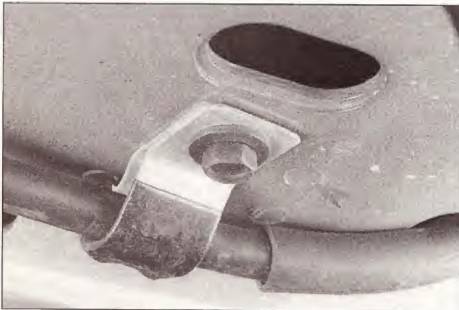
10.12d ... remove this cable bracket bolt (arrow) from the underside of the pan, ...
