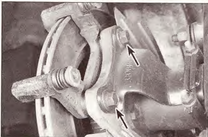
5.7b Rear caliper anchor plate bolts (arrows)
