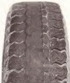
INCORRECT TOE-IN OR EXTREME CAMBER
