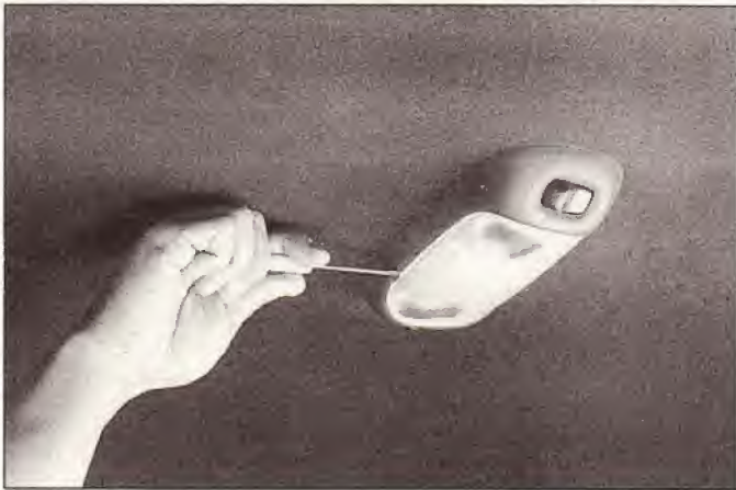
18.17 Use a small screwdriver to pry out the interior light lens
