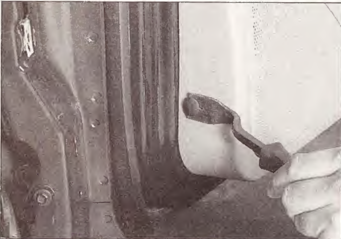
17.5 Detach the plastic clip (arrow) securing the front edge of the door trim panel
