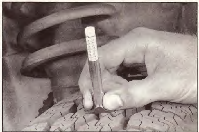
5.2 Use a tire tread depth indicator to monitor tire wear - they are available at auto parts stores and service stations and cost very little
