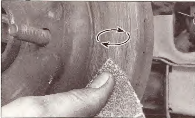
5.5b Using a swirling motion, remove the glaze from the disc with sandpaper or emery cloth
