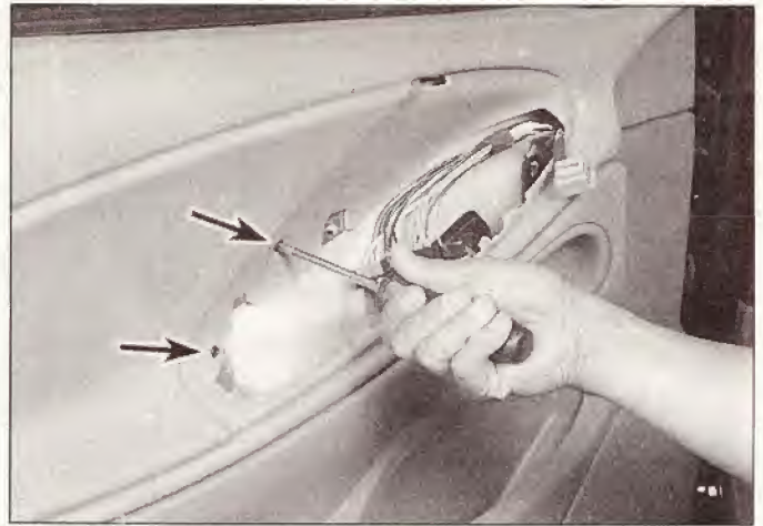
17.4 Remove the retaining screws (arrows) located behind the armrest switch control plate
