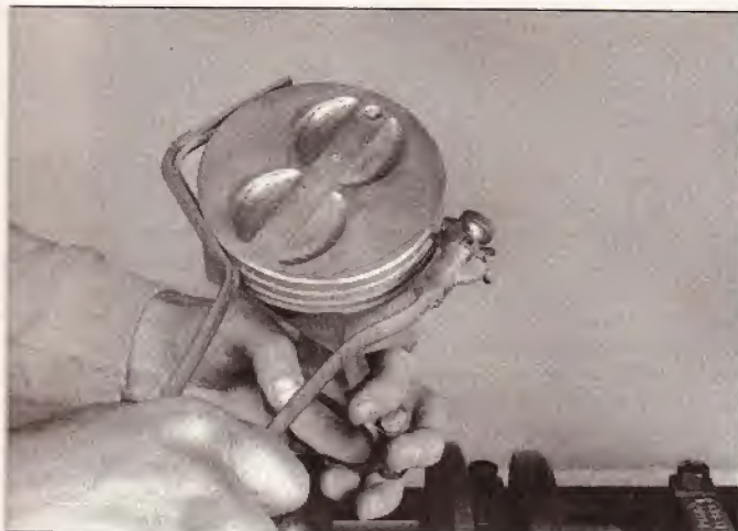
18.4a The piston ring grooves can be cleaned with a special tool, as shown here . . .
