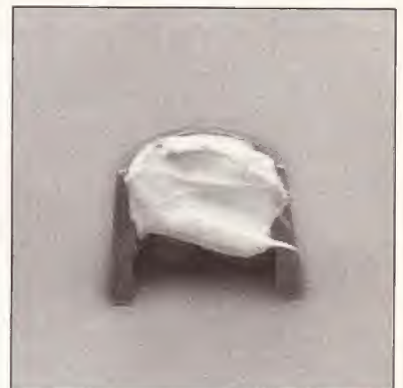
10.22 Apply a small dab of grease to each keeper as shown here before installation - it'll hold them in place on the valve stem as the spring is released
