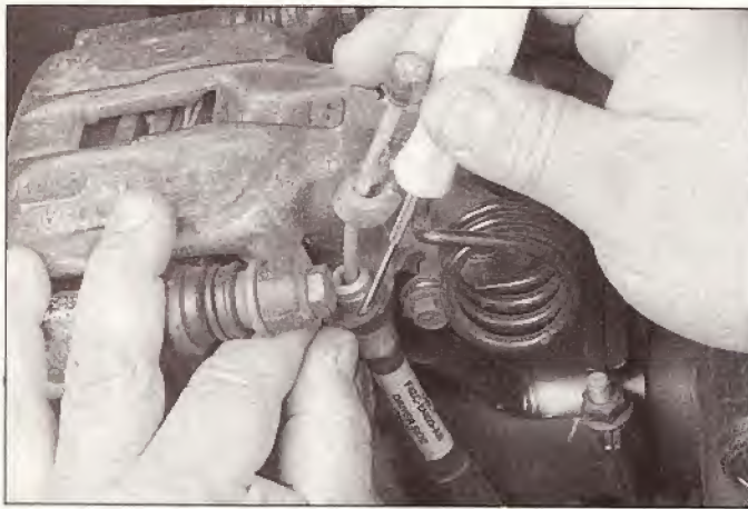
10.12b ... remove this C-clip from the cable boss on the rear caliper, ...
