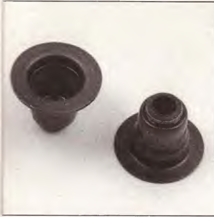
10.20a The valve stem seals combine a seal with the valve spring seat
