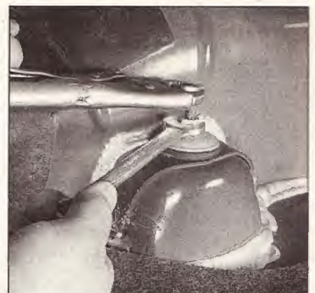
10.3 Locate the upper retaining nut for the shock absorber inside the trunk; to prevent the piston rod from turning, hold it with a wrench or locking pliers while you break loose the nut
