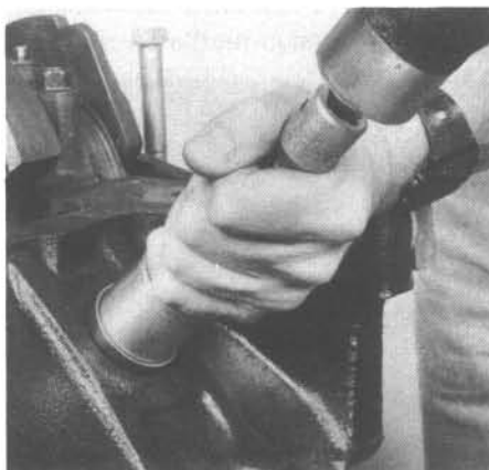
14.10 A large socket on an extension can be used to drive the new core plugs into the bores
