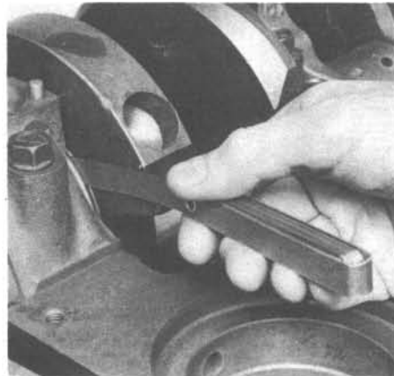
13.3 Checking crankshaft endplay with a feeler gauge
