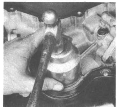
16.8 Clean the bore, then apply a small amount of oil to the outer edge of the new seal and drive it squarely into the opening with a large socket and a hammer – don't damage the seal in the process and make sure it's completely seated
